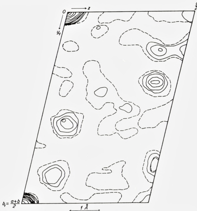
Fig. 3. Patterson projection on (1\bar{1}0) . Relative arbitrary scale.
